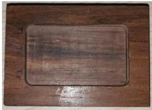
Figure 9. Surface cutting results with a spindle speed of 8000 RPM
