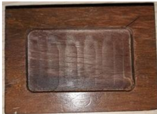
Figure 7. Surface cutting results with a spindle speed of 4000 RPM
