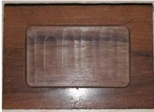
Figure 8. Surface cutting results with a spindle speed of 6000 RPM
