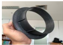
Figure 4. Narrow paper core problem with core plug on the side
