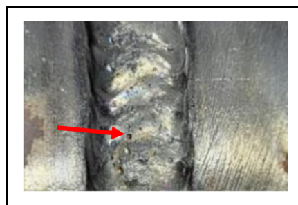
Figure 2. Surface cluster porosity
