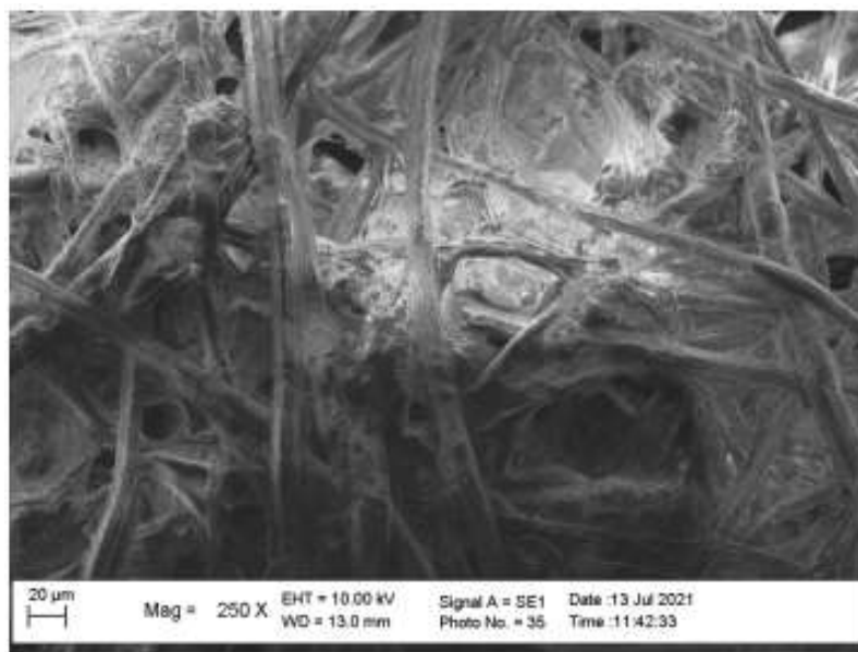
Figure 2. SEM measurement results of palm fiber-based paper with 250x magnification
